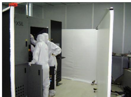
Both are 1.92 m (6 ft 4 in) high, which is high enough to protect the eyes of anyone less than 6 ft 8 inches tall standing right up to the screen, while low enough to pass through a standard doorway. The screens can be made higher if desired.
