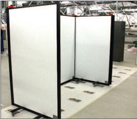
The screens consist of a 50 mm thick sandwich of steel and a special lightweight laser-blocking material, with a white laminate finish on both sides. This is mounted on a powder-coated steel framework, with heavy-duty lockable castors.
