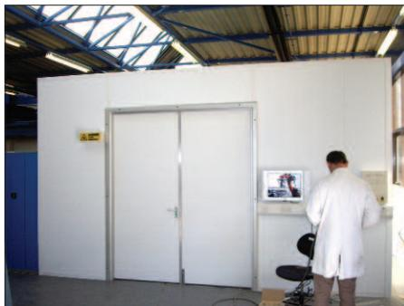
Laser enclosure with interlock system and CCTV
