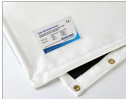
The material is fireproof. When irradiated with greater than 0.5 MW/m<sup>2</sup> it will emit a non-hazardous smoke and may glow, thus indicating that a stray beam is present. Protection times given by the material at various power densities are shown in the specifications below.
