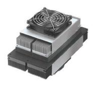
The AA Outdoor Cooler Series is an air-to-air thermoelectric assembly (TEA) that uses impingement flow to transfer heat. It offers dependable, compact performance by cooling objects via convection. Heat is absorbed and dissipated thru high density heat exchangers equipped with air ducted shrouds and brand name fans. The heat pumping action occurs from custom designed thermoelectric modules that achieve a high coefficient of performance (COP) to minimize power consumption.
