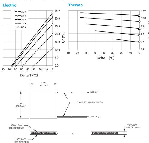
Ceramic Material: Alumina (Al<sub>2</sub>O<sub>2</sub>)
