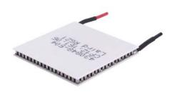
The ZT Series is a high performance thermoelectric module (TEM). The module I assembled with premium Bismuth Telluride semiconductor material that achieves a higher temperature differential than standard single stage TEMs.
