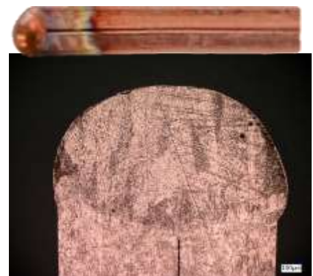
Figure 3. Top Image highlights the uniform spherical shape and heat affected zone generated from the process. Bottom image is a cross section showing no porosity or defect within the welded area.
