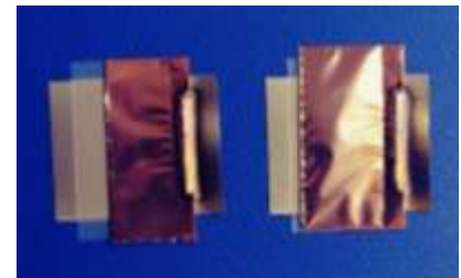
Figure 3. Cu Foil Welded to Ni-coated Cu Tab
