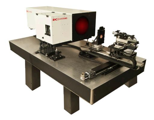
CI Systems offers a cost effective and modular optical test bench to measure the Modulation Transfer Function (MTF) and transmission of optical components in the visible, SWIR, MWIR and LWIR spectral ranges. The OptiShop allows for video and slit scanning MTF tests.
