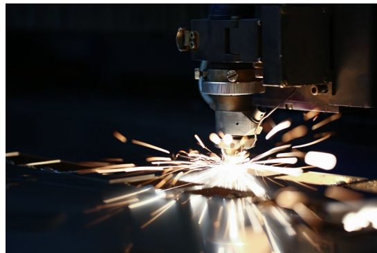
Industrial lasers used for cutting hard materials require a cooling solution to ensure stability of the laser beam.
